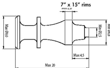
The stud dimensions for ice tyres mounted on a 7" x 15" rim are as follows:
